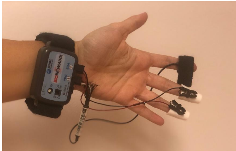
Figure 9: Placement of the BIOPAC sensors on the participant's fingers.
