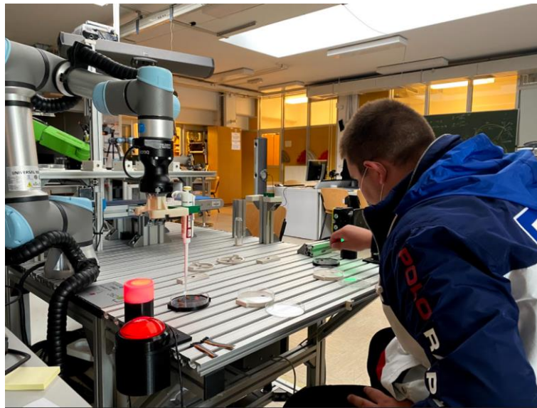
Figure 4: Operator placing filter paper discs on the petri dish while the robot is preparing a new batch of paper discs soaked with antibiotic dilution.
