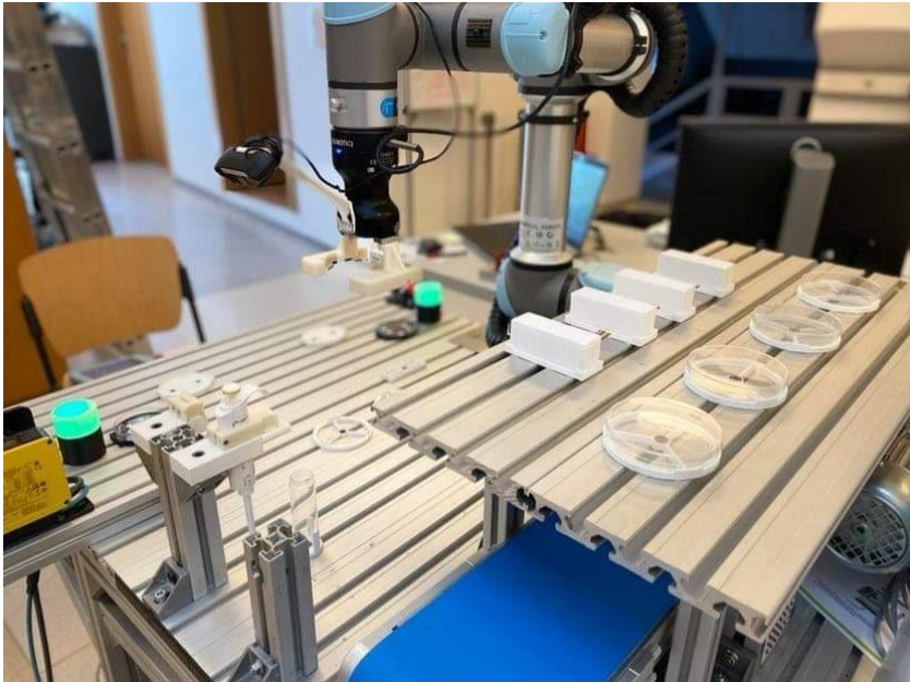
Figure 4: Shared working area of the participant and the robot.
