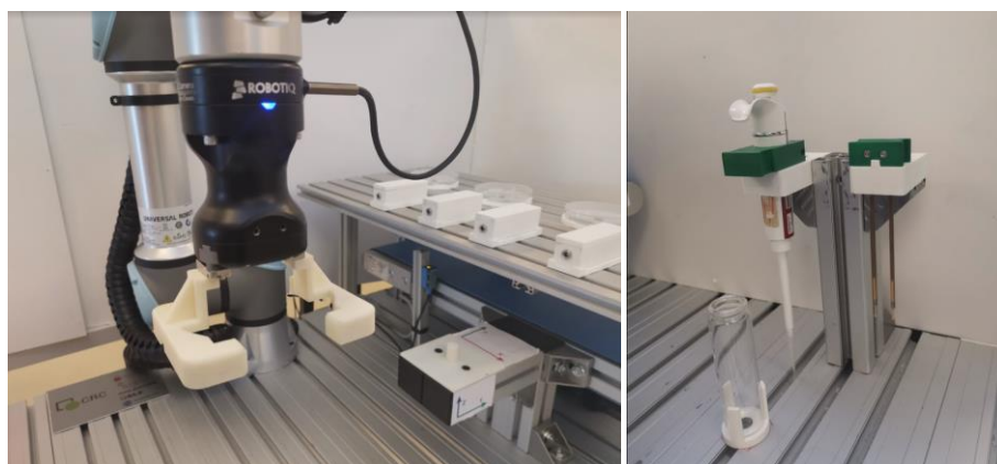
Figure 1: Robot's gripper with 3D printed fingers for gripping box enclosure/petri dish - safe tool (left), and testing leads and pipette - dangerous tool (right)
