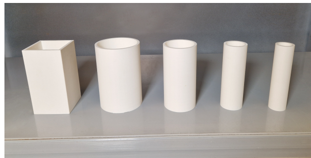
Figure 8. The reference objects of different shapes and sizes. From left to right: flat object with 80 mm side, curved object with radius 100 mm, curved object with radius 75 mm, curved object with radius 50 mm, and curved object with radius 37.5 mm. All objects have a height of 150 mm.
