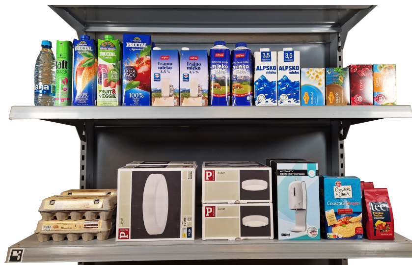
Figure 6. The experimental setup of retail shelves. Objects are positioned in a dense configuration to emulate real retail store conditions.
