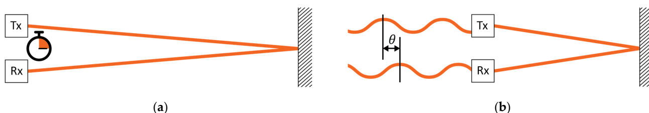
Figure 1. Principle of operation of (a) direct and (b) indirect time of flight measurement.
