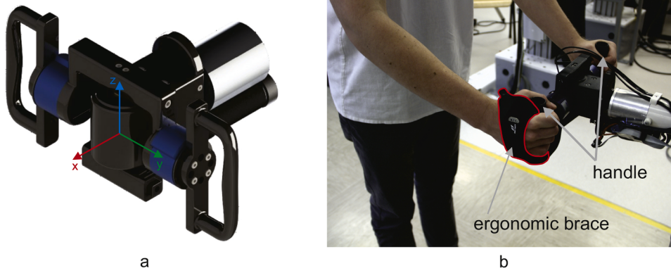
Fig. 2. The figure shows an instrumented handle system with two F/T sensors—one for each hand—and its local coordinate frame. Rotations occur about the X-axis (subfigure a). Subfigure (b) shows how participants place their hands on the instrumented handle with attached ergonomic brace (annotated with red border).
