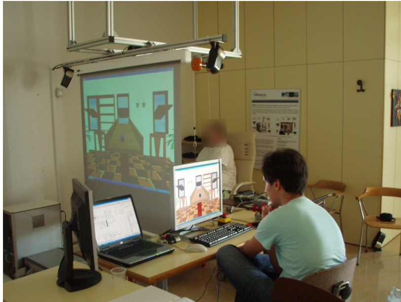
Figure 3.9: The room where the experiment took place. The task was displayed on a large screen using backprojection (middle left). The subject (center, blurred for anonymity) sat in front of the screen. The robot (not visible) was situated between the subject and screen. A metal frame (top) supported the screen, speakers and gravity compensation motors. The experimenter (lower right) sat to the side and had access to a secondary task display screen (lower center) as well as a separate computer used for physiological recordings (lower left).
