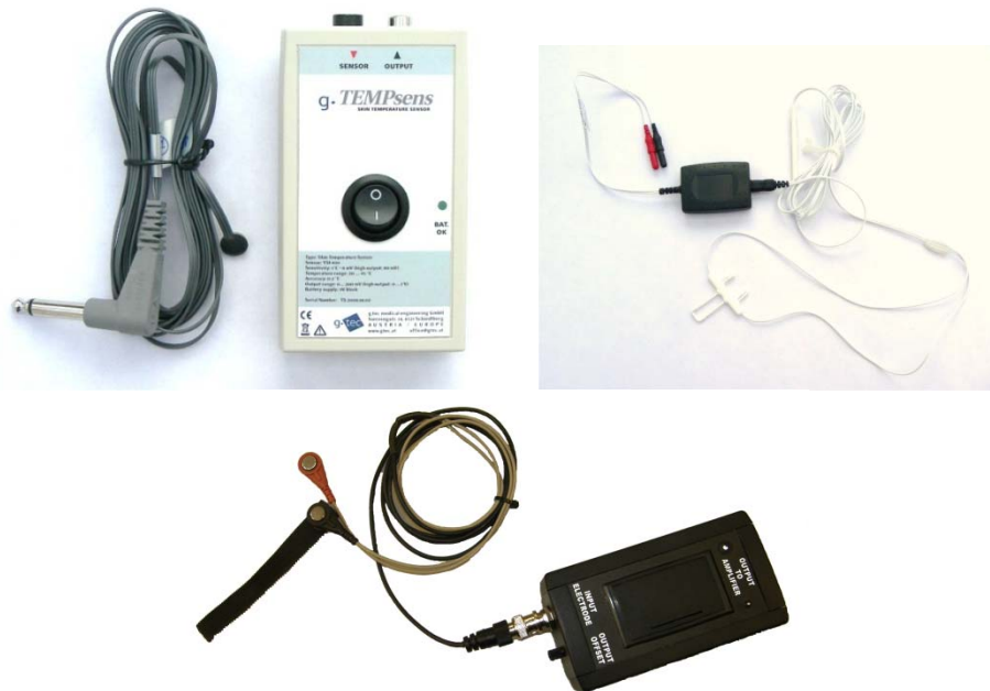
Figure 2.4: Physiological sensors: temperature (top left), respiration (top right) and skin conductance (bottom). All manufactured by g.tec.
