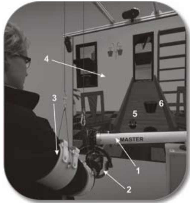
Figure 3: A subject performing the task using a haptic robot (1) and grasping device (2) while his/her arm is supported by cuffs (3). The screen (4) shows a sloped table, a ball (5) and a basket (6).
