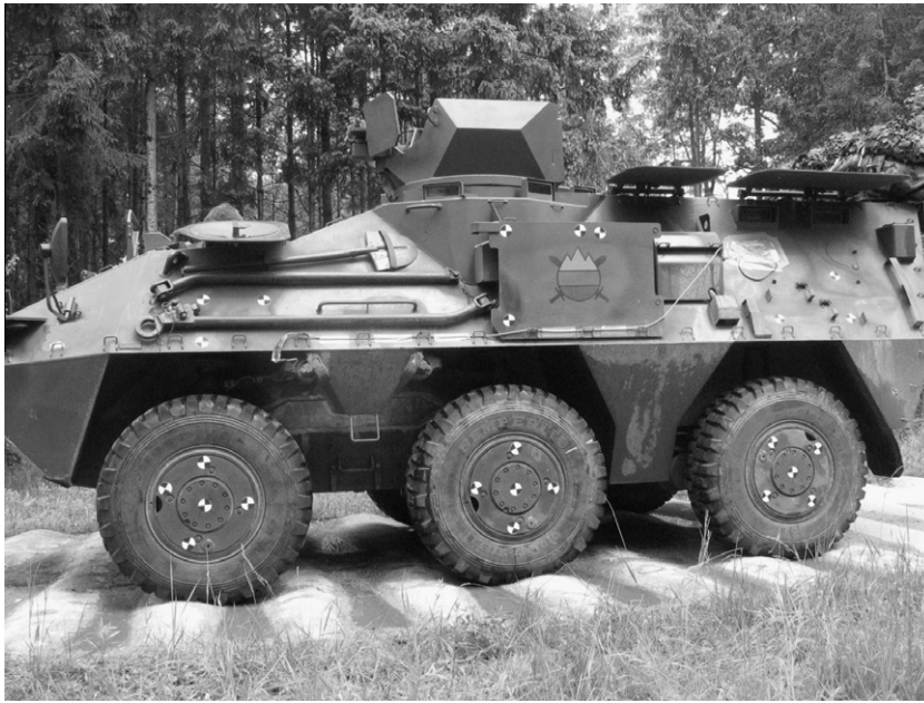
Fig. 13. Vehicle under test on the “washboard” test track.
