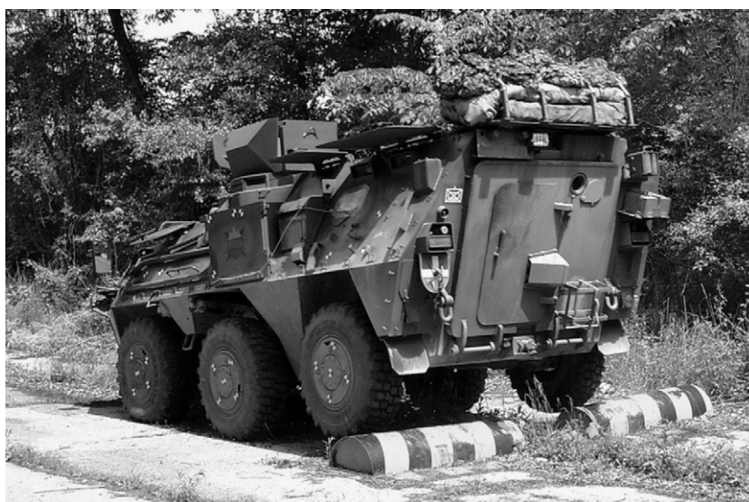
Fig. 12. Vehicle under test on a half-cylinder test track.
