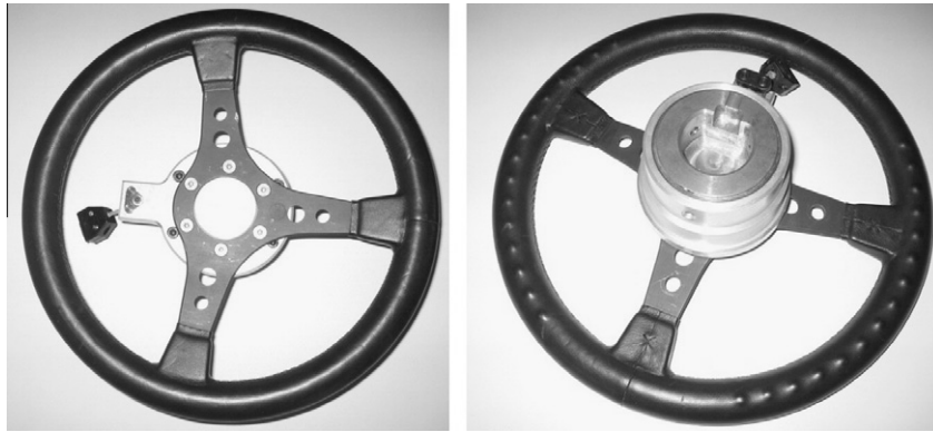
Fig. 18. Device for measuring the steering wheel torque.
