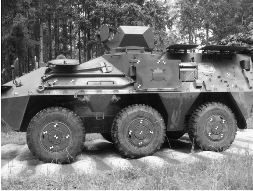
Fig. 13. Vehicle under test on the “washboard” test track.
