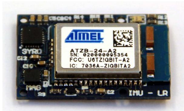
Fig. 1. IMU that consists of a three-axis gyroscope, a three-axis magnetometer, and a three-axis accelerometer and a wireless module with a dual-chip antenna. The size of the IMU is 30 \times 20 \times 5 mm without a battery.
