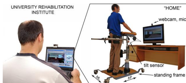
Figure 1. Diagram of proposed tool. The physiotherapist can supervise, control, and monitor a patient's targeted balance training in the VE in real-time. The physiotherapist and the physician can check the outcomes remotely and provide necessary instructions to the patient via teleconference. The therapeutic goal was the weight transfer from the unaffected to the affected side extremity, and thus the speed of the movement in the VE was proportional to the tilt of the balance frame.
