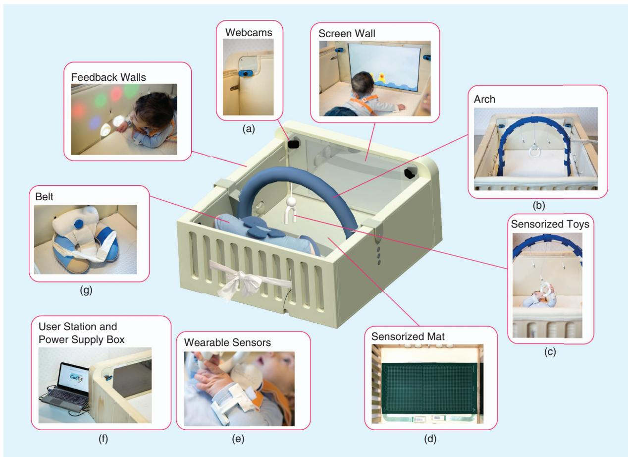
**Figure 1.** The CareToy platform and its components: (a) the box with interactive walls (lights, sounds, and four webcams), (b) an arched gym, (c) four sensorized toys, (d) a sensorized mat, (e) three wearable sensors (two bracelets and a chest strap), (f) a user station (laptop for the parents or operator) with a power supply box, and (g) a sensorized belt. (Photos courtesy of The BioRobotics Institute.)
