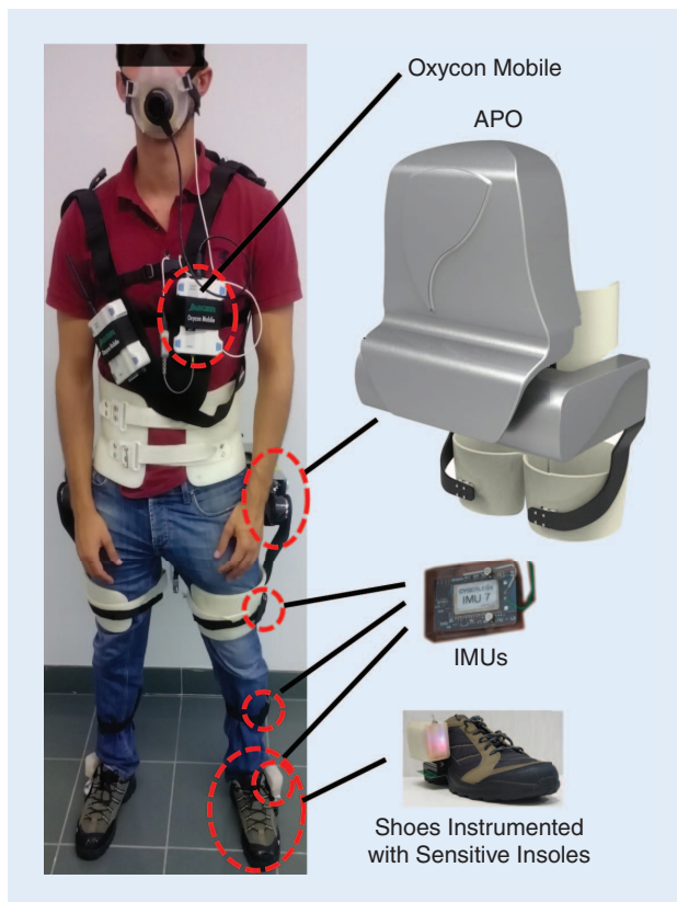
Figure 4. The frontal view of a person wearing the experimental setup. The following components are visible: Oxycon Mobile, APO, the sensory system with IMUs, and the shoes instrumented with custom pressure-sensitive insoles. For more details on the latter two, see [30]. (Photos courtesy of Virginia Ruiz Garate.)
