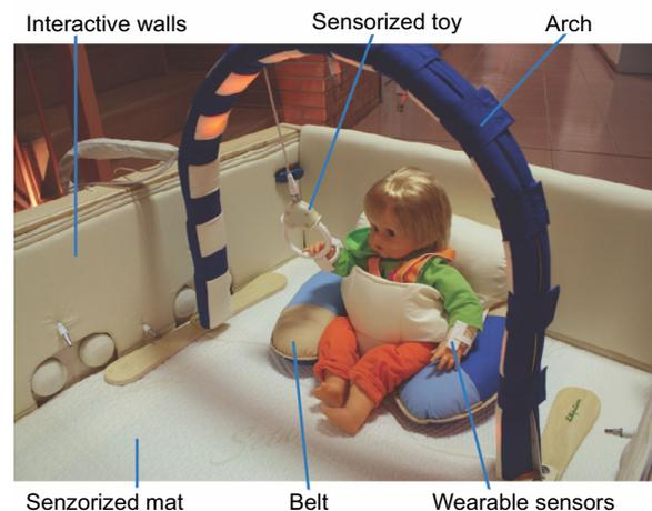
FIGURE 1. CareToy platform and its main modules, which are indicated with text and blue lines.
