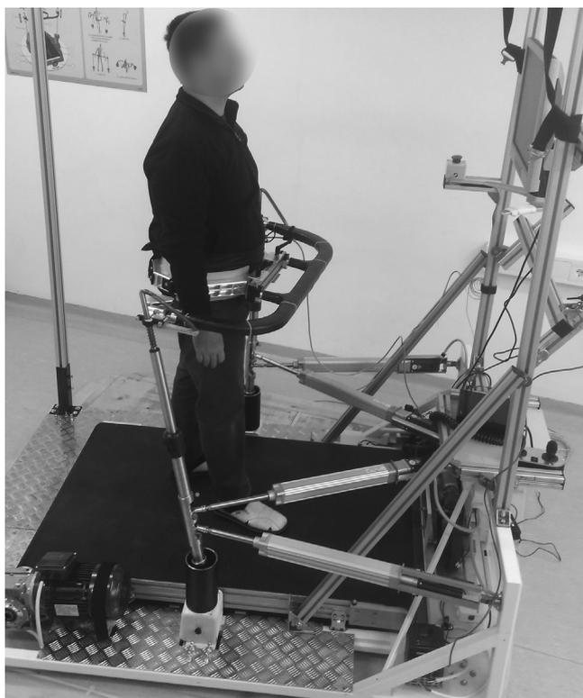
Fig. 1. Photo of a subject walking on an instrumented treadmill while being embraced by the BAR perturbing device (up). Top view illustration of perturbation directions (down).
