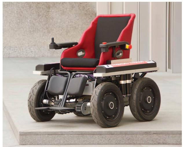
**Figure 1.** A robotic wheelchair with a wheel-track design.
