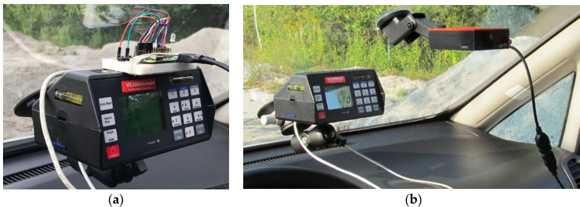
Figure 5. (a) Breadboard prototype on the calibrated measurement device during initial testing; (b) Finished prototype and the calibrated measurement device mounted on the vehicle windshield, ready for brake testing.
