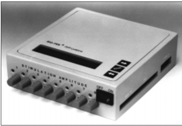
Fig. 1. Eight-channel functional electrical stimulator.
