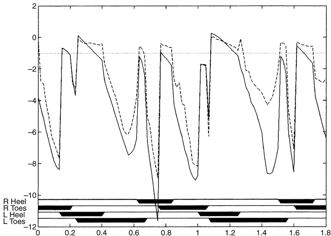
**Figure 3.** Static/kinematic gait stability in an above knee amputee as assessed by the wearable system (dashed line) and offline by VICON motion analysis system (solid line). Basogram in the bottom depicts gait phases, the dotted line divides stable and unstable region.
