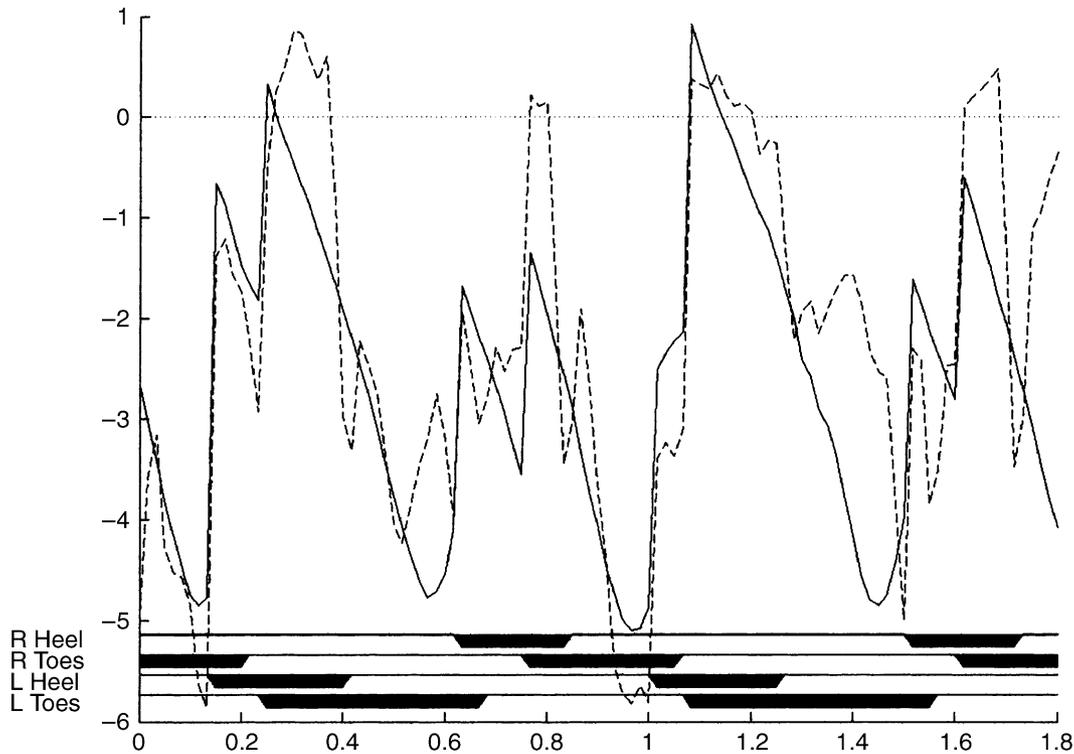
**Figure 4.** Dynamic gait stability in an above knee amputee as assessed by wearable system (dashed line) and offline by VICON motion analysis system (solid line). Basogram in the bottom depicts gait phases, the dotted line divides stable and unstable region.
