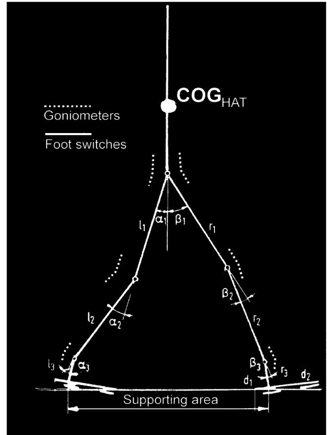
**Figure 2.** Wearable system setup: goniometers at main leg joints and foot switches under both feet.
