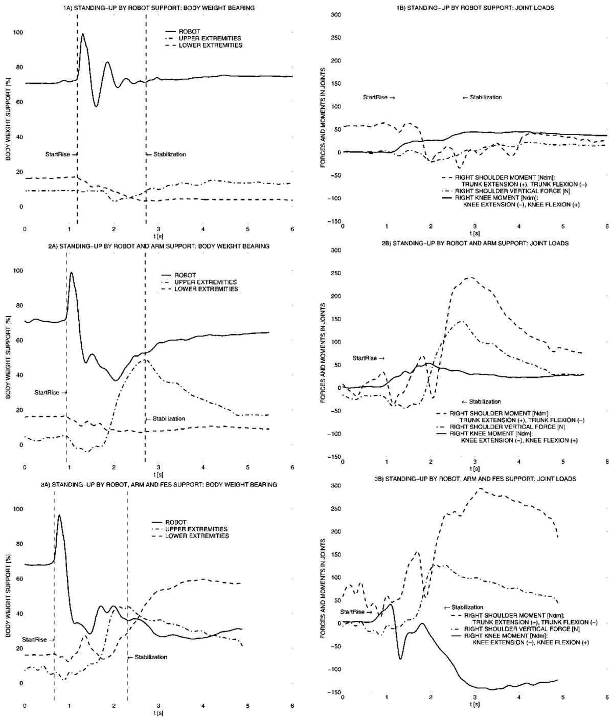
Figure 4. Bodyweight bearing and joint loads during: (1) robot-assisted standing up, (2) robot- and arm-assisted standing up, and (3) robot-arm and FES-assisted standing up.
