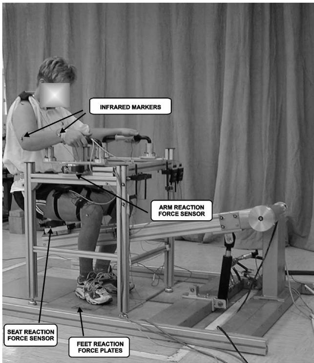
Figure 3. Paraplegic subject and the standing up measurement setup.
