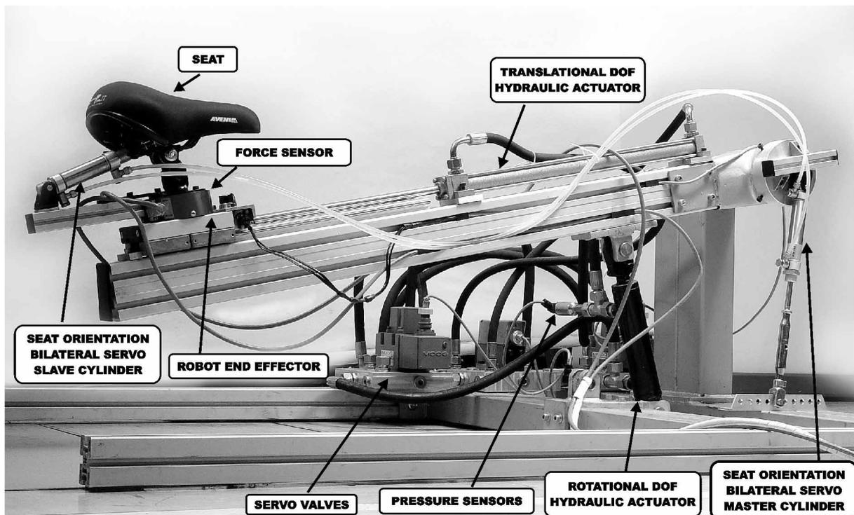
Figure 1. Standing-up robotic supportive device.
