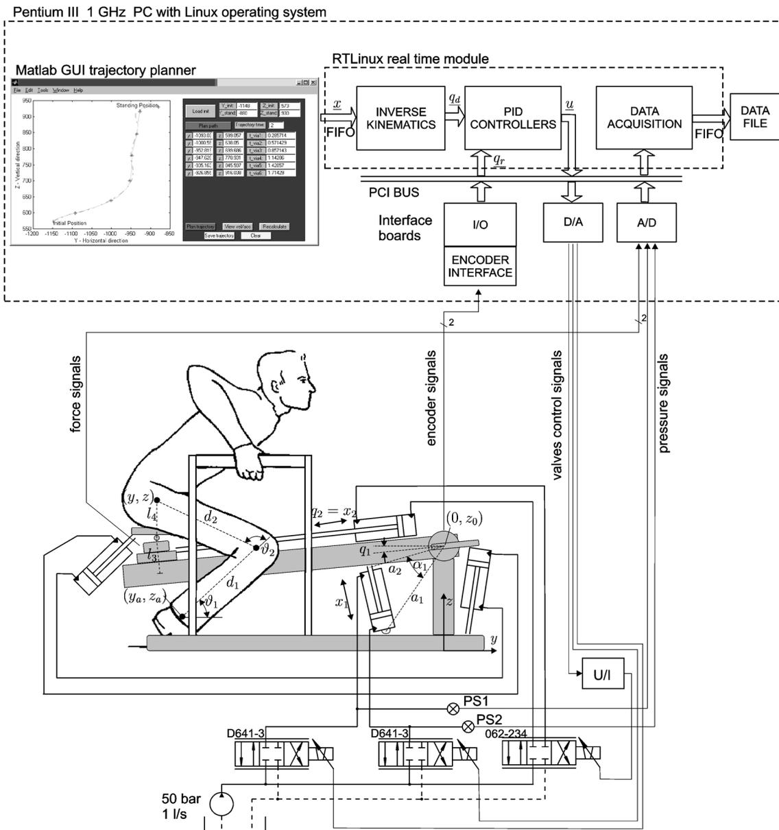
Figure 2. Control system of the standing up robotic assistive device: hydraulic circuit diagram, trajectory planner and real-time controller.
