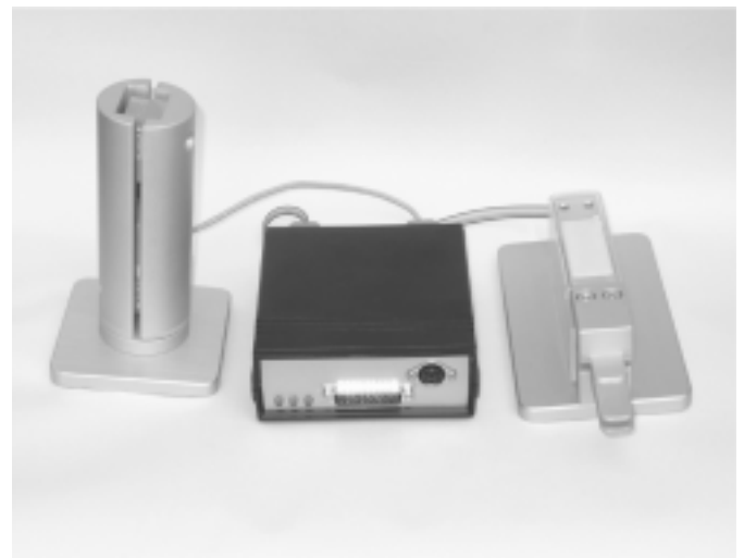
Figure 1. A compact assessment system with two different measuring objects in the shape of a cup and thin plate can be connected to a personal computer to accurately measure the dynamic grip force in cylindrical and lateral grip.
