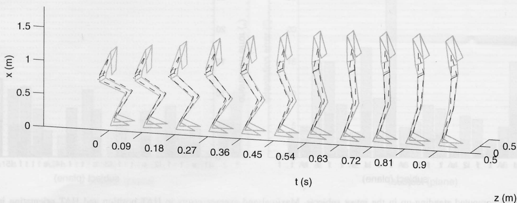
Fig. 3. Measured (solid line) and computed (dashed line) standing-up of the intact person II. The computed HAT is represented by the triangle; right hip—center of mass—left hip.
