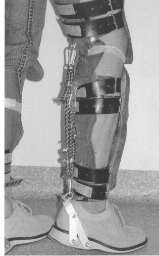
Figure 1 — Schematic and photograph of a participant during walking with emulation of SOL and GAS muscle contracture. The system consists of trousers with leather patches sewed on the inner side and two fixation rings corresponding to proximal ends of SOL and GAS muscles, shoes with aluminum framework carrying fixation ring corresponding to distal ends of SOL and GAS muscles, and elastic ropes, representing emulated muscle contractures.
