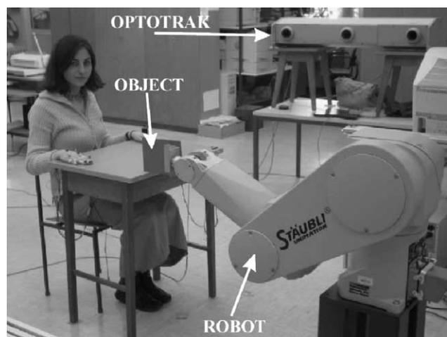
Fig. 1. The object presented to the subject by a robot. Movement was recorded with the OPTOTRAK system.
