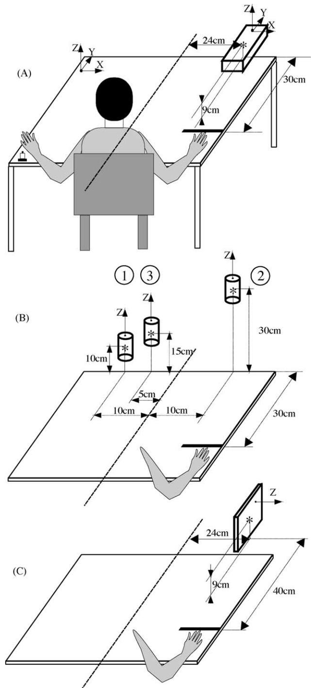
Fig. 2. Experimental set-up: positions and orientations of the block (A), cylinder (B), and plate (C) (\* signifies the object COG).
