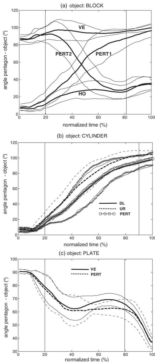
Fig. 7. Average angle trajectories between pentagon and object normal ( $\pm$ S.D.) for (a) block, (b) cylinder, and (c) plate. Vertical lines represent start and end-point of object perturbation.
