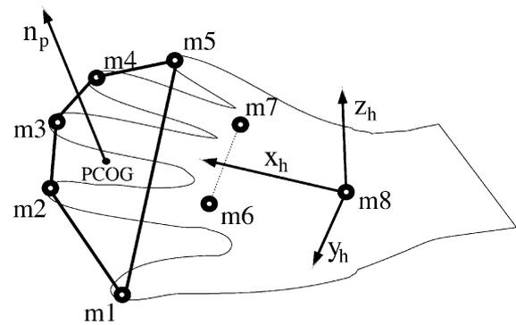
Fig. 4. Position of eight markers on the tips of the fingers and dorsum of the hand. The pentagon connecting the finger markers is characterized by its center of gravity (PCOG) and normal  $n_p$ .  $(x_h, y_h, z_h)$  represents hand coordinate system.
