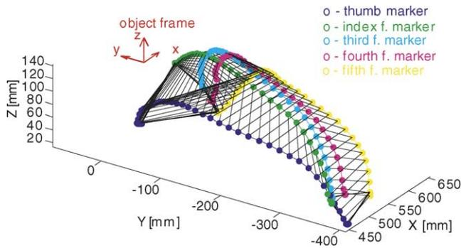
Fig. 3. Trajectory of the fingers pentagon during the reaching-to-grasp movement.
