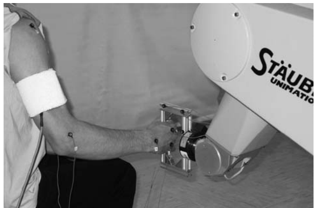
Figure 5 Experimental setup—robot Staubli RX90B with JR3 force sensor, inertial system attached to the upper arm, and OPTOTRAK infrared markers on the arm, hand, and robot handle.
