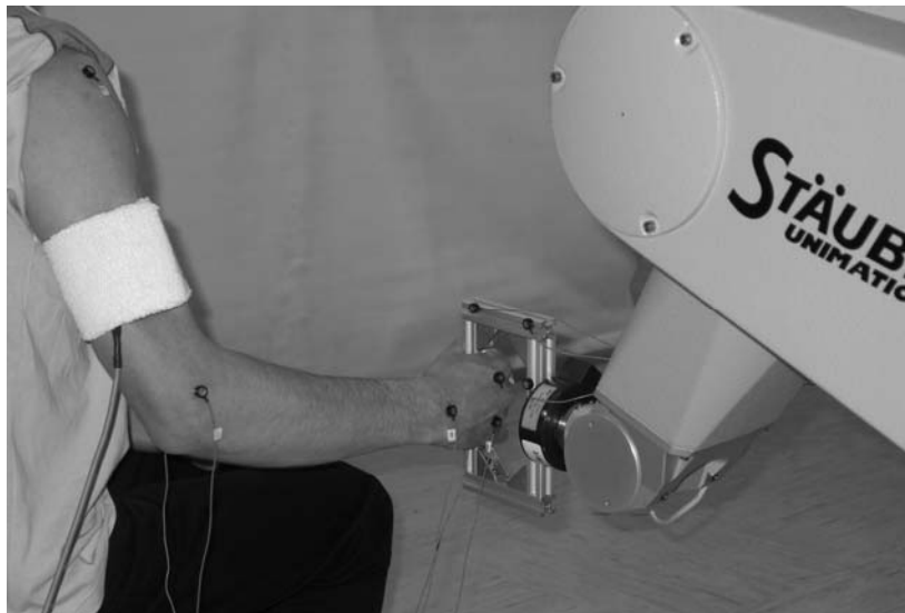
Figure 3 Experimental setup: robot Staubli RX90B with JR3 force sensor, accelerometers attached to the upper arm, and OPTOTRAK infrared markers on the arm, hand, and robot handle.
