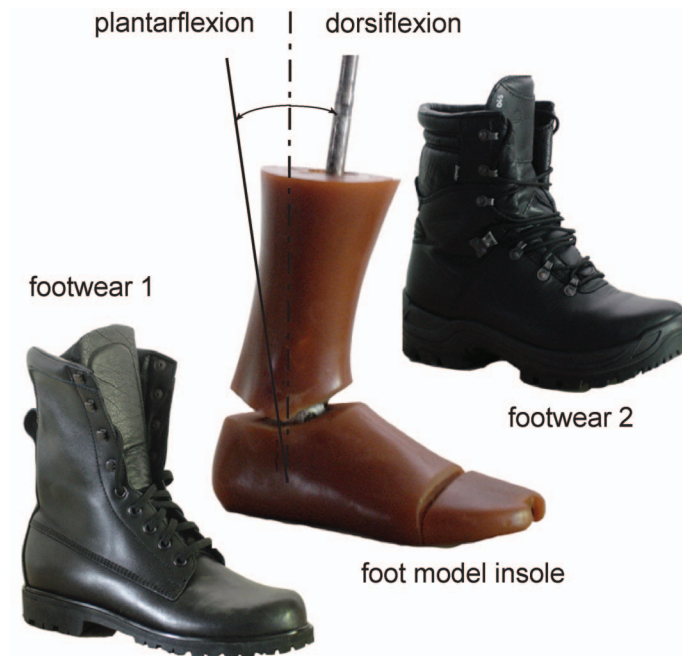
Figure 1. Prototype boots used in the study. A foot model with flexible ankle joint in all three planes was used to assess boot stiffness in selected angles of stance phase.
