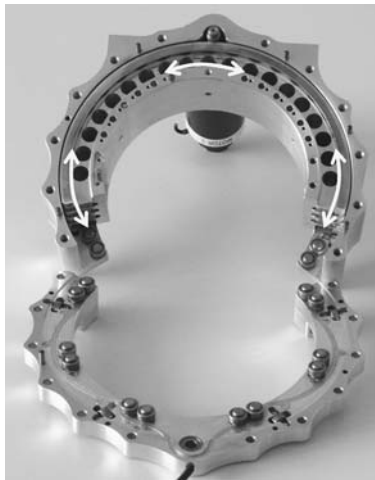
Fig. 2 Upper arm rotary module for internal/external shoulder rotation (opened to allow view inside)
