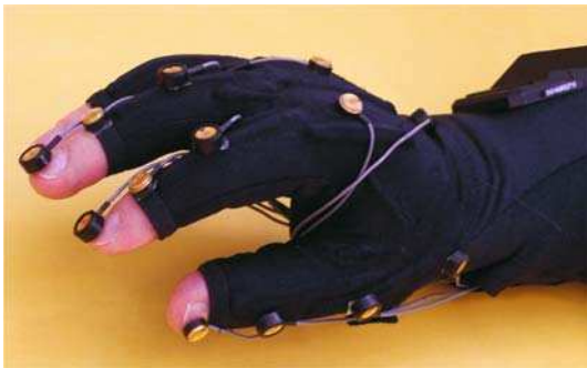
Fig. 2 Measurement set-up: instrumented glove and infrared markers attached to anatomical landmarks above the CMC, MCP, PIP, DIP, and IP joints, to the capitate bone, and on the fingertips
