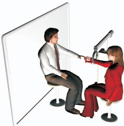
Fig. 4. Virtual physiotherapist experimental setup - 3D projection screen (white) with a virtual physiotherapist projected in 3D, HapticMaster robot with haptic grasping device, patient doing exercise with the virtual physiotherapist.
