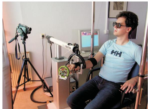
Fig. 1. Subject training with HEnRiE: a grasping device is attached to the HapticMaster end-effector, a 3D projection screen is positioned in front of the subject, a thin Kevlar wire connects the elbow cuff with the arm gravity compensation motor positioned above the subject.
