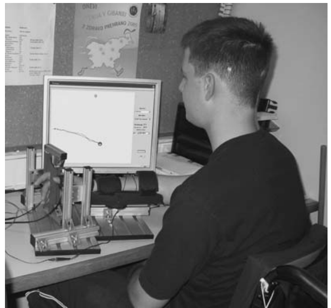
FIGURE 3. Incomplete tetraplegic subject accomplishing the force training task with the system for upper extremity sensorimotor augmentation.
