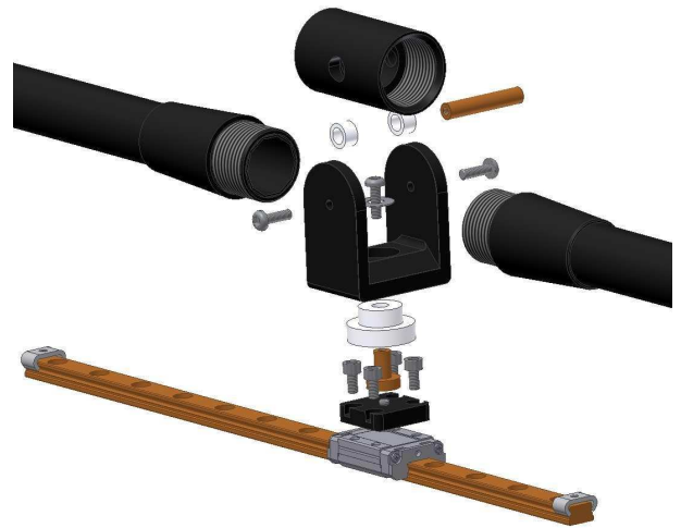
Figure 1. Exploded view of a 3-DOF joint placed in the middle of the mechanical extension. The joint consists of two rotational DOFs and one linear DOF
