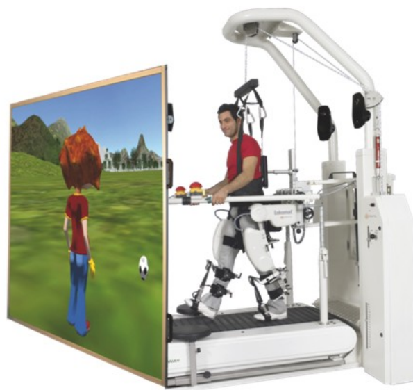
Fig. 3. Robotic gait orthosis Lokomat including visual and auditory displays.
