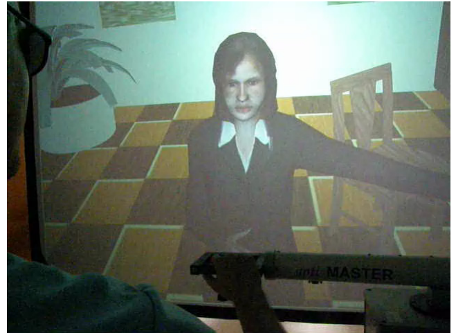
Fig. 6. Virtual physiotherapist experimental setup - 3D projection screen (white) with a virtual physiotherapist projected in 3D, HapticMaster robot with haptic grasping device, person doing exercise with the virtual physiotherapist.
