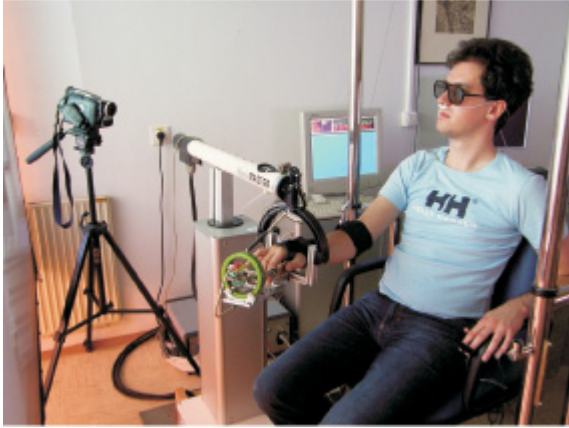
Fig. 4. Subject training with HEnRiE: a grasping device is attached to the HapticMaster end-effector, a 3D projection screen is positioned in front of the subject, the elbow cuff links to the arm gravity compensation motor positioned above the subject.
