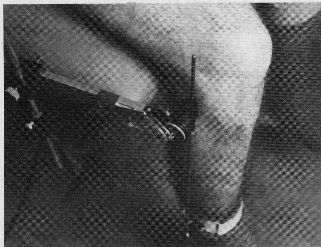
Figure 3 Oblong hole in potentiometer axis, allowing free movement of the joining bar, perpendicularly to the sagittal plane and in proximal-distal direction
