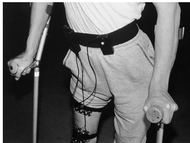
FIG. 3. This photograph shows an incomplete tetraplegic patient walking with the assistance of a 2-channel stimulator and the telemetry system. The receiver module and the stimulator are tied to the patient's waist.
