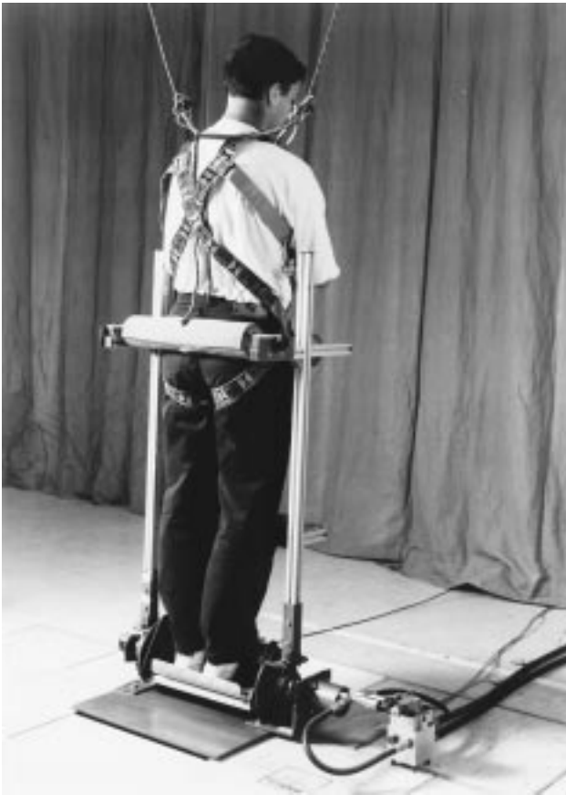
Fig. 3. An intact subject standing in the MRF. The restraining aluminum beams, standing platform and safety ropes are clearly shown. The hydraulic actuator and incremental encoder are also visible.
